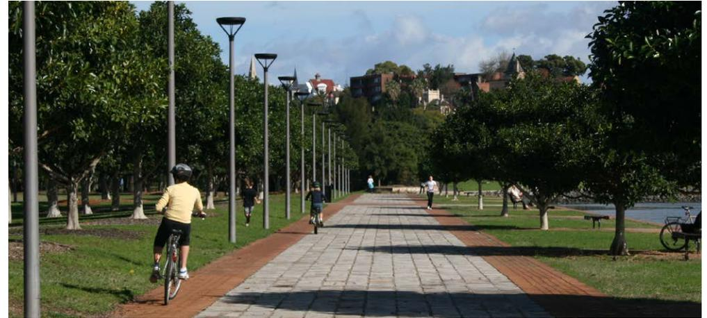
Shared path designed to manage speed and interaction using surface treatments on the Glebe Foreshore in Sydney, NSW
