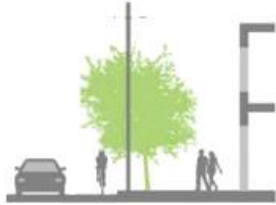
Small tree under powerlines
