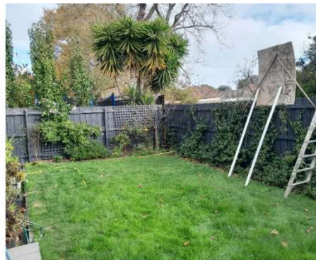
Fig 5. Southerly view of backyard (SPOS), with pseudo wall installed for shadow testing. 2pm shadow measurement, with yellow tape 4.2m from fence.
