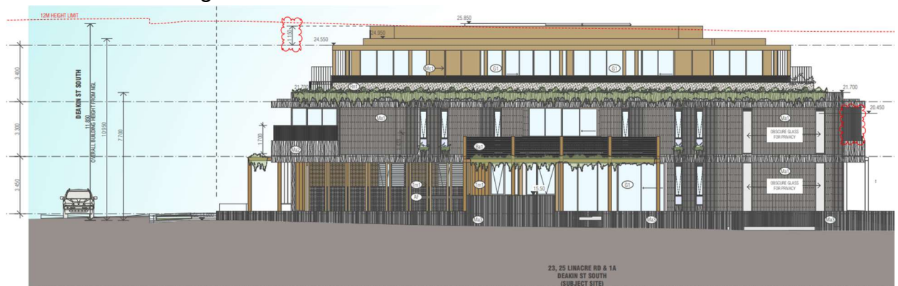
Fig 1 - TP202 showing 12m building height breached
