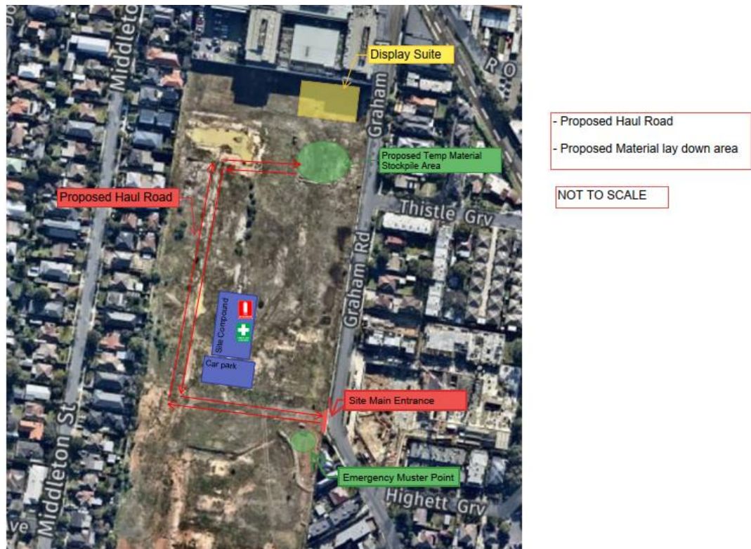
Figure 3 Proposed Site Compound and Display Suite Location
