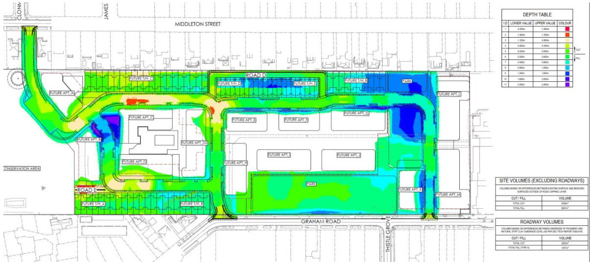
Figure 6 Bulk Earthworks Plan - Cut and Fill
