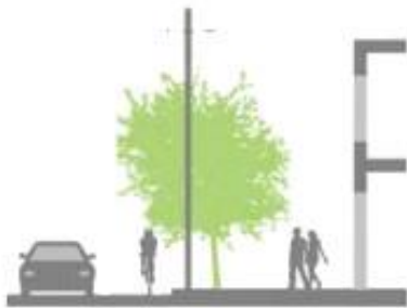
Small tree under powerlines
