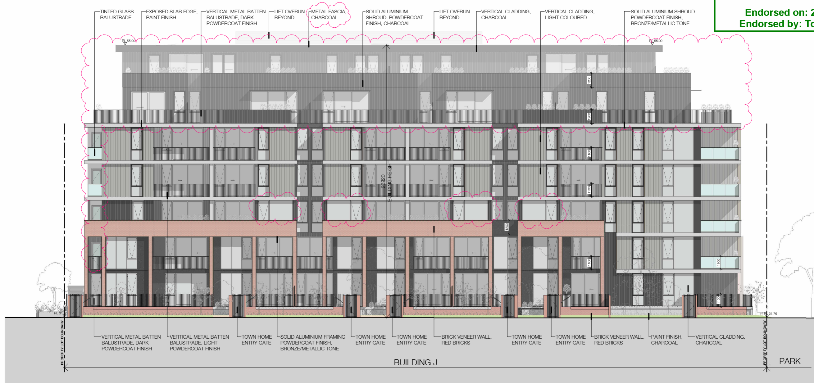
Building J - East Elevation
